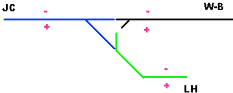
We've determined that when the track switch is thrown from Jersey City to Wilkes-Barre, we want the Allentown block to be normal (ground on the wall side, hot on the aisle side). With the track switch thrown from JC to WB, you determine that relay contacts 6 & 7 and 9 & 10 are making contact. Since we want the track to be 'normal' we'll need to connect contact 7 to the big ground wire, and contact 10 to the block toggle on the panel.
