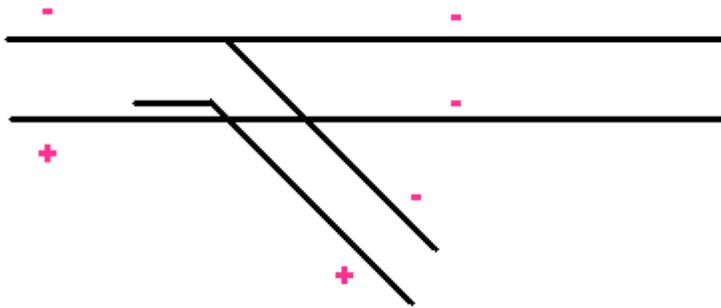
If the switch points are touching the rail closest to the wall, then the top contact that is touching the tab gets wired to same wire as the back rail (usually the ground wire).
