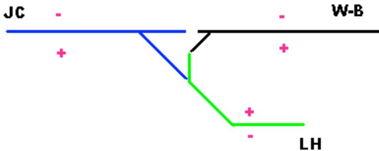
When we throw the track switch to route the train from Lehigh to Wilkes-Barre, we'll now need to reverse polarity. That means we'll wire contact 5 to the block toggle and contact 8 to the big ground wire. Viola! The polarity is changed when you throw the switch machine.
