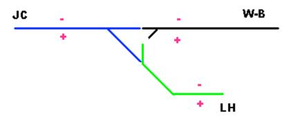
We've determined that when the track switch is thrown from Jersey City to Wilkes-Barre, we want the Allentown block to be normal (ground on the wall side, hot on the aisle side). With the track switch thrown from JC to WB, you determine that relay contacts 6 & 7 and 9 & 10 are making contact. Since we want the track to be 'normal' we'll need to connect contact 7 to the big ground wire, and contact 10 to the block toggle on the panel.
