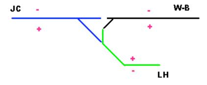
When we throw the track switch to route the train from Lehighton to Wilkes-Barre, we'll now need to reverse polarity. That means we'll wire contact 5 to the block toggle and contact 8 to the big ground wire. Viola! The polarity is changed when you throw the switch machine.
