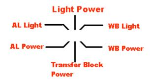
These toggles also differ in the way they're physically wired. One side of the physical toggle connections carry block power, while the other side of the toggle carry the blinking light power.
